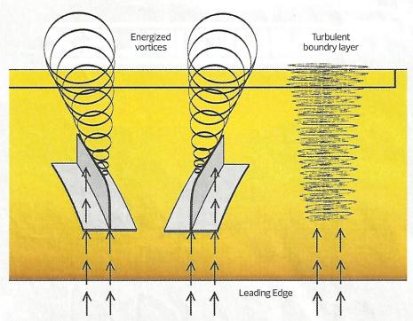
Vortex generators are positioned obliquely (e.g., 10-20 degrees) so that they have an angle of attack with respect to the oncoming airflow (thus causing the airflow to spill over eachVGand form the highly energized vortex).
