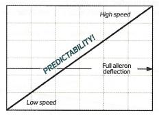
Thicker control surfaces with round leading edges help the airflow remain smooth and attached to the control surfaces when deflected for maximum control authority at all airspeeds. Thicker control surfaces with round leading edges achieve a smoother airflow over them and therefore provide greater stability and a more even (linear) control response starting from neutral.
