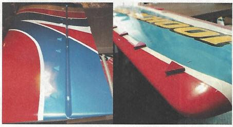
significant impact! Because of this, we use thicker control surfaces and/or vortex generators on every airplane in the flight school training fleet. They improve each pilot's ability to maintain positive control at slow speeds and in wind, as well as tame the tip-stall tendencies of certain models. Most important, thicker control surfaces
