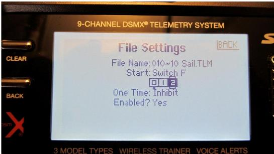
I have to pull switch F all the way down (position 2) to start recording
