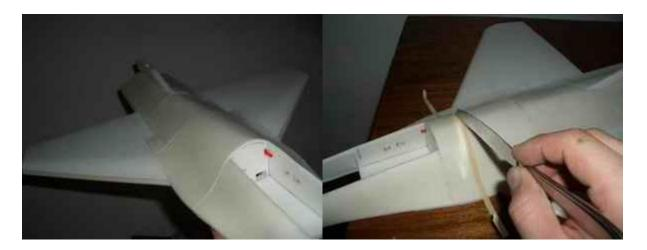
Cut out the vertical fin and sand some profile in it. Score rudder hingelines etc. Wait with installing untill the last possible moment.
