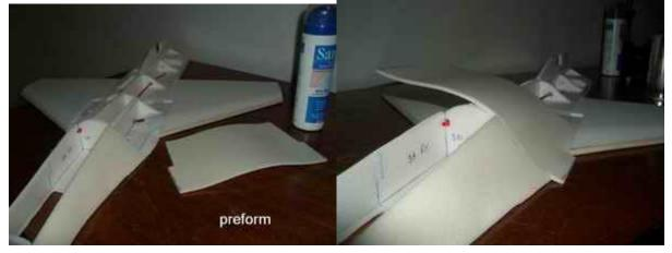
If you have beveled the bottom plate enough before, the wing / fuselage joint will be nice and smooth.
