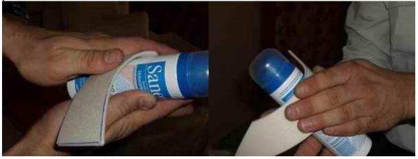
Cut the LH and RH cockpit sheeting. Preform it with a spraycan and your fingers. Glue the top first. When that is cured put glue on the formers and bottom plate. Spray some accelerator in there and fold it down. Hold with your hands untill cured.
