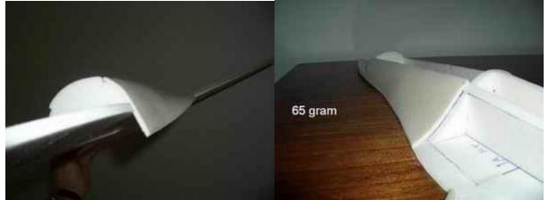
Cut the fwd middle top sheeting using the template. Prefom and trial fit again a lot of times to make sure it fits properly. If you do, there is no need for filler and the lines will just look like original panel lines. Start with glueing one side. Then the other.
