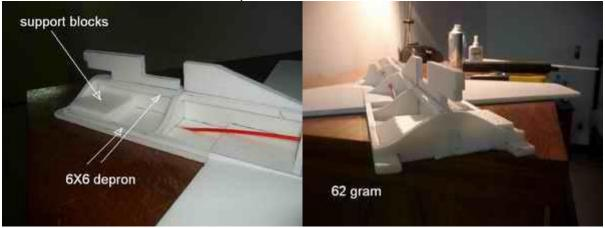
Prepare the nose section for sheeting. Draw a line from former 3D to the next fwd. Check the cross sections of these formers to see where to bevel the baseplate piece 1A. Bevel from 6 to 0 mm. Use sandpaper to bevel fuselage next to wingroot. You want to go 3 mm deep so that when you glue the top sheeting on the fuselage, the sheeting will be flush with the wing. See pictures.
