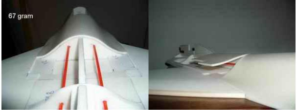
Cut the aft middle sheeting. Preform and trial fit. Check the blue line to see what you try to achieve. After the thickest point in the wing the aft fuselage is perpendicular to the wing, this was also already achieved during the wingprofile sanding process and now you add 3 mm sheeting to it
