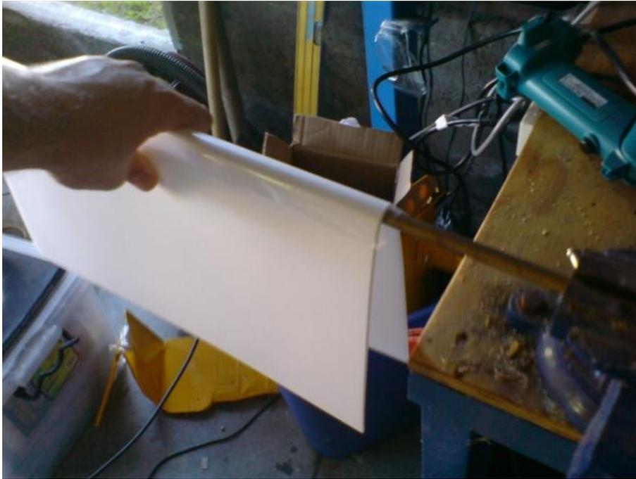
5. Glue the trailing edge with your glue of choice. I use UHU foam glue or hot melt. They both work well. Push the spar into the wing sideways, then twist it upright to pop the wing into shape. Repeat the process for the other wing.
