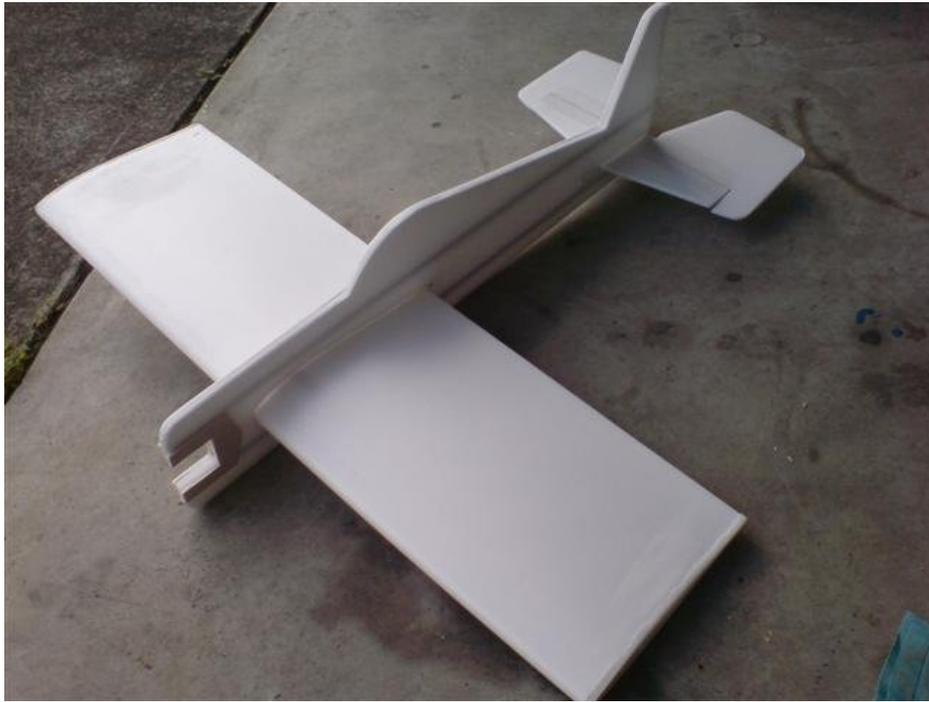
Next tape on the ailerons using the same method as you did for the elevator. CA hinges could be used for all control surfaces if you preferred.
