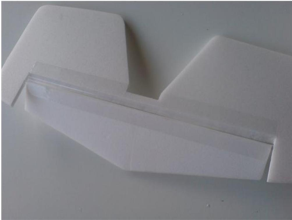
Attach the rudder using CA hinges then add end caps to the wings. 6mm Depron is best for this. Cut out the end caps to fit inside the ends of the wings, not like these photos where I capped the outside of the wings. You will get a much better finish when you come to sand them.
