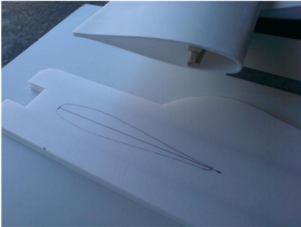
Fit the wings. Take your time with this part. It's the hardest bit of the build. Make sure the wings are level, and then glue them in place using 5 mins epoxy. You can use hot melt if you like, or both. Finish the join with a bead of glue where the wing and fuse meet.
