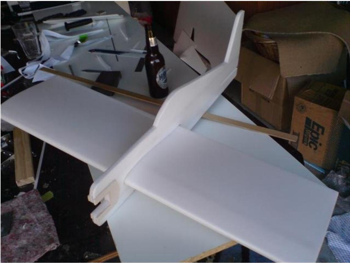
7. Time to make the horizontal stab and elevator assembly.
