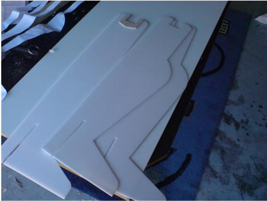
Take the 6mm section and use a hot soldering iron to make channels for the carbon spars.
