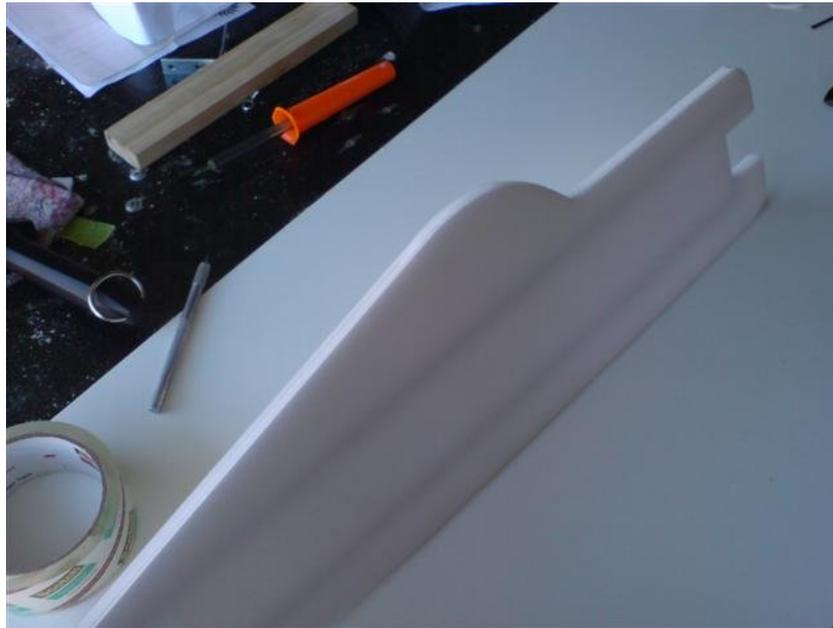
Trim the trailing edges of the wings square, fit the spar and mark the wing leading and trailing edge location from the plan onto the fuse. Next use the wing to trace around and draw the outline onto the fuse. Cut out a hole to fit the wings into.
