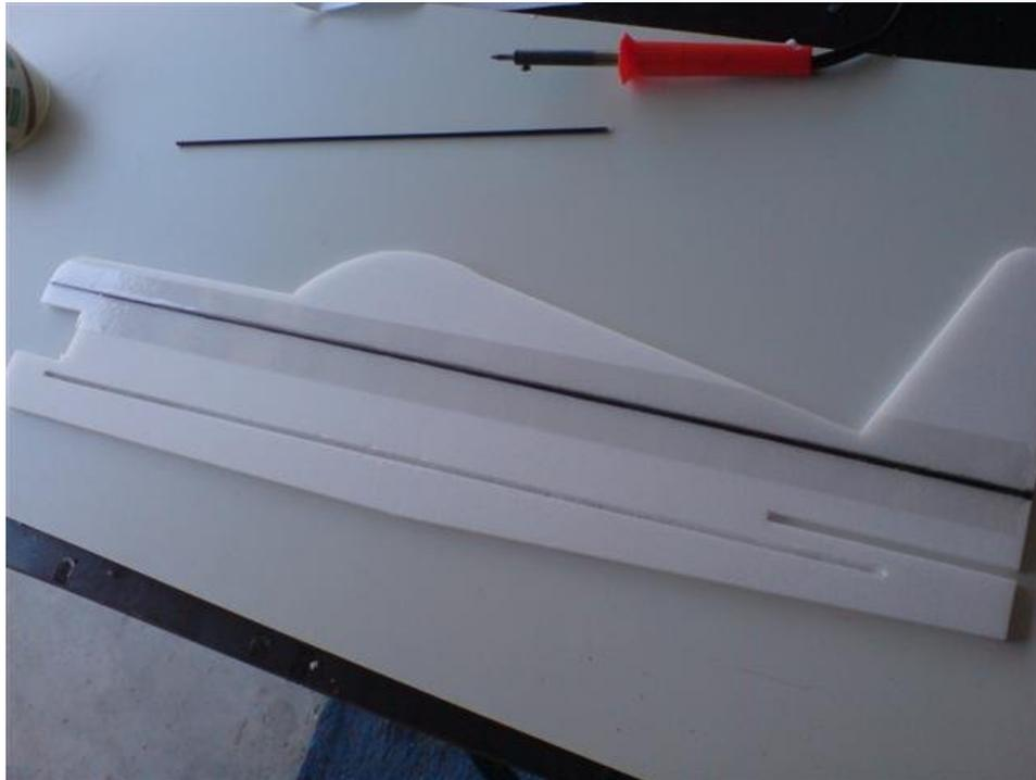
Now Glue the skins to the outside to produce a nice stiff 12mm thick Fuselage.
